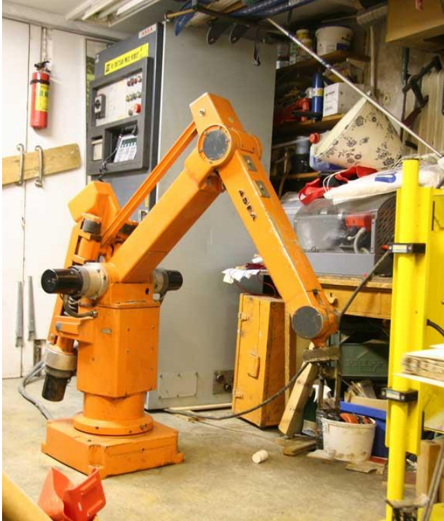
ABB IRB 6 (1973) first commercially available all electric micro- processor controlled robot
