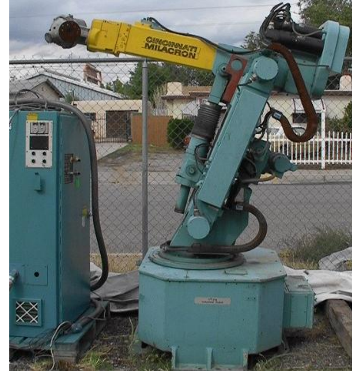
Cincinnati Milacron T3 (1974) first micro-computer controlled robot
